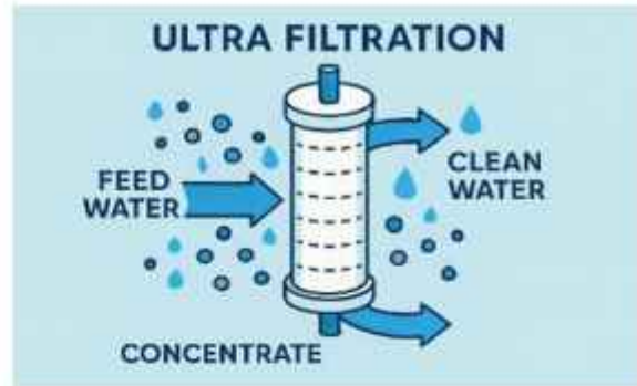
Figure: 12 UF Purifiers (Picture Courtesy Google)
